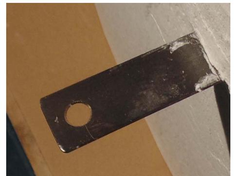
Easily bolted, strip leads are sized to accommodate the current draw of each custom-made RDI heating element. Strip sizes range from 1mm(0.04") to 3mm(1.3") thick x 12.5mm(0.5") to 25mm(1.0") wide.
