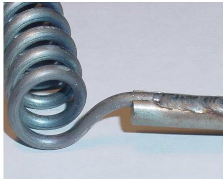
Solid rod leads with or without threaded ends are securely mig-welded to the FeCrAl resistance wire. Welded leads are stress-annealed before the RDI heating element assembly is vacuum-formed.
